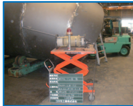
鋼板製曲管φ2,600mm X線検査
